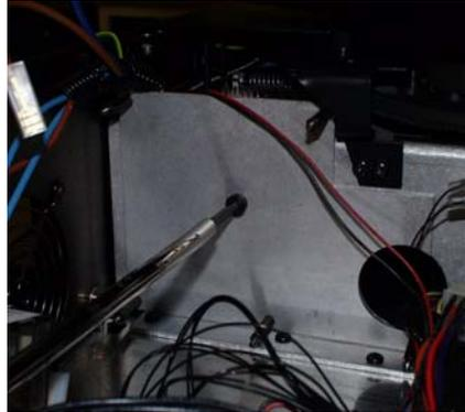
*Fig. 2 Remove screw from bracket*
